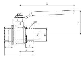
DN shows the nominal flow diameter. Actual flow diameter complies with full port DIN 3357 part 4. Stem configuration of valves over 2" is slightly different.
